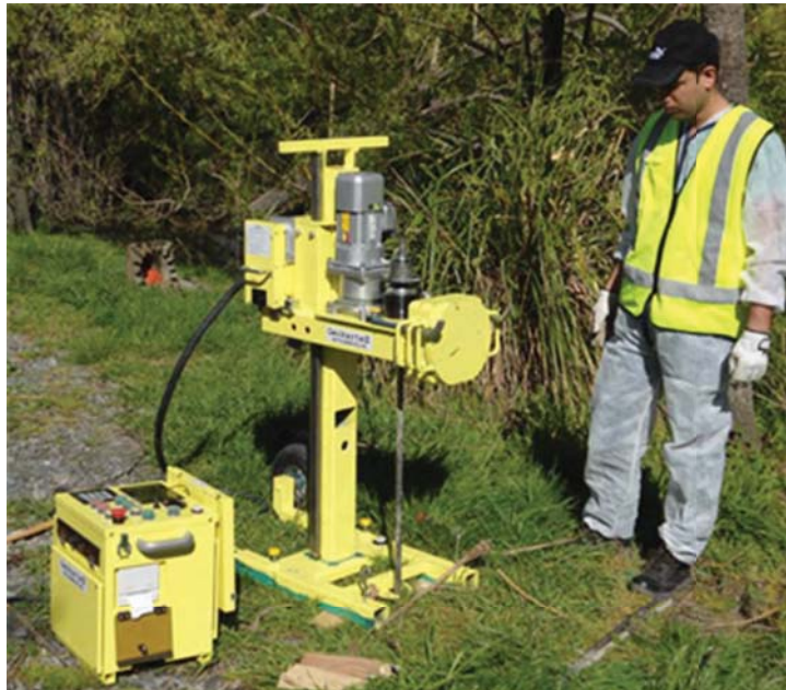
Figure 3. Screw driving sounding (SDS) equipment.
