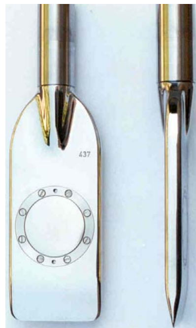
Fig. 1. The flat dilatometer - Front and side view
