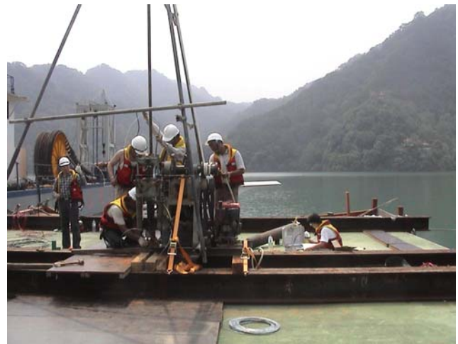
Figure 8. Operation of TDR/DMT from a barge.
