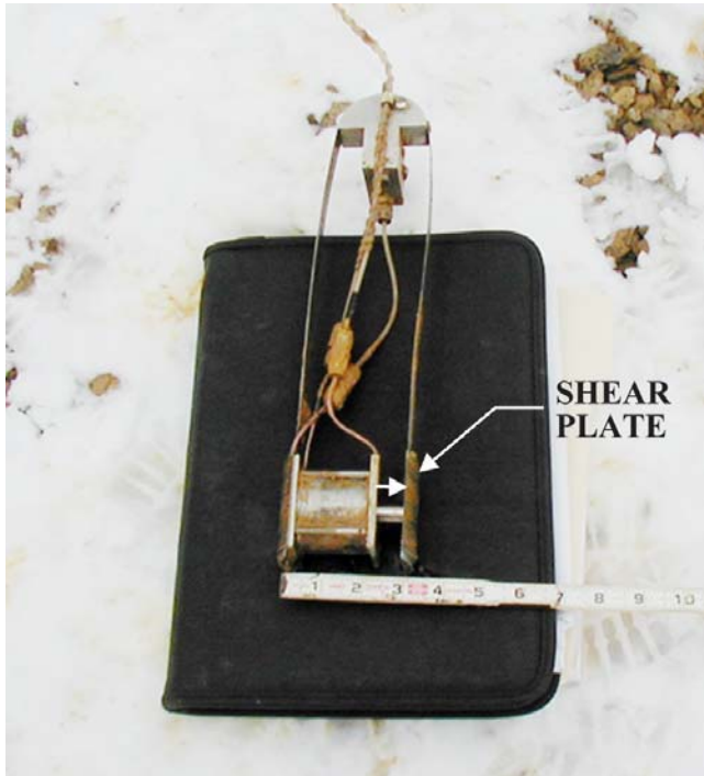
Figure 11. View of borehole shear head with shear plate in expanded position
