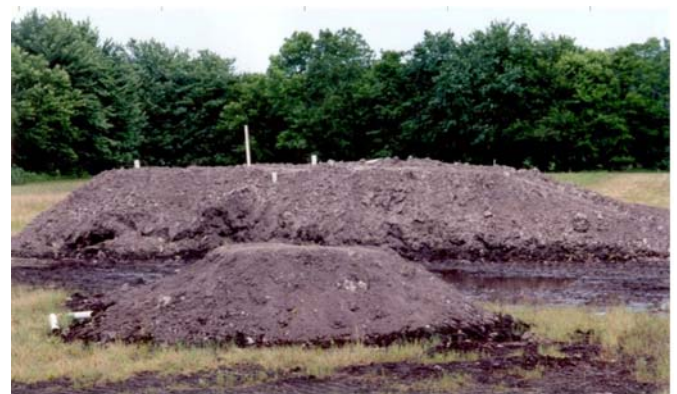
Figure 6: Embankment load test setup
