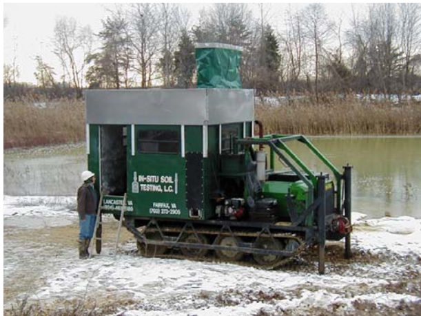
Figure 8. Track-mounted DMT rig.
