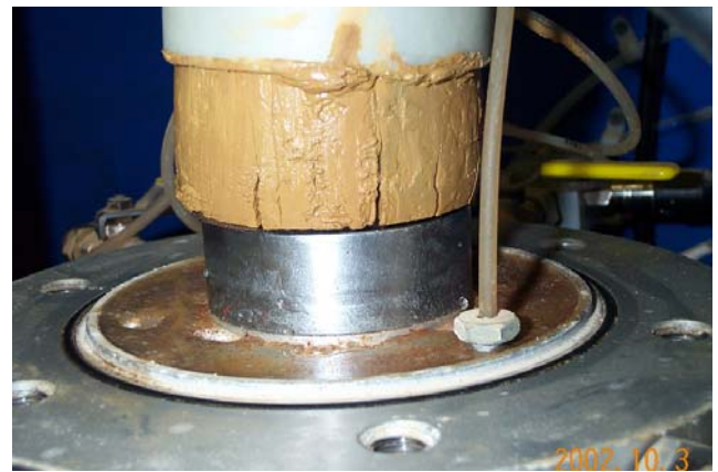
Figure 7. Sample of clayey washings expanding due to lack of confinement during extrusion from Shelby Tube.
