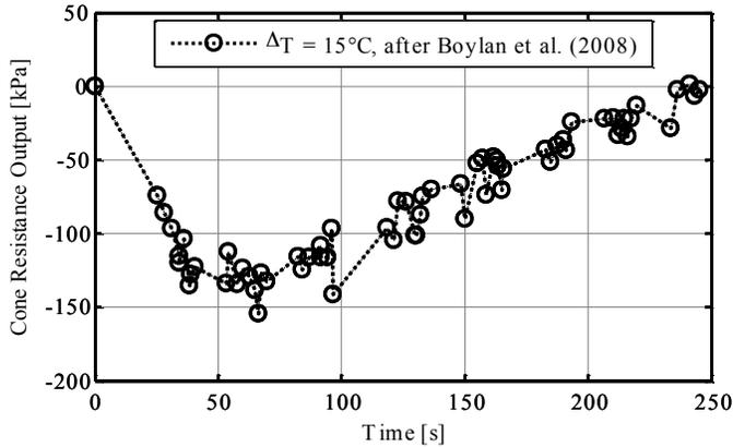
Figure 8. Laboratory variation of  $q_c$  upon transient temperature differential (Boylan et al. 2008).
