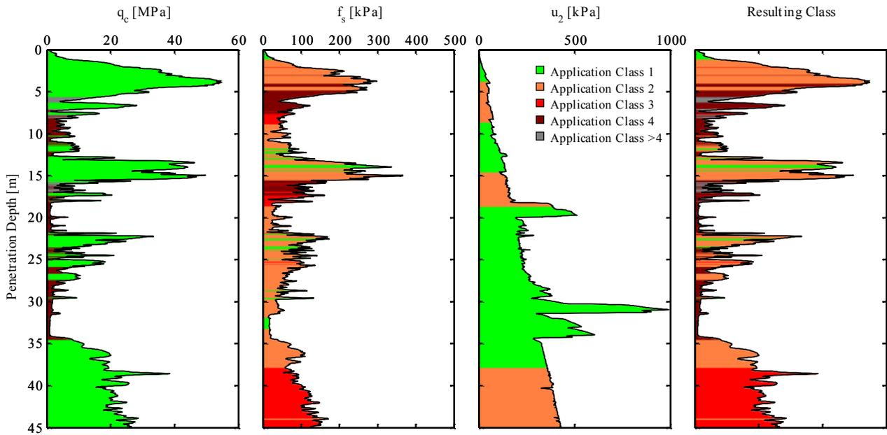
Figure 20. Demonstrating compliance to ISO application classes, for adverse conditions of layered sands and clays.
