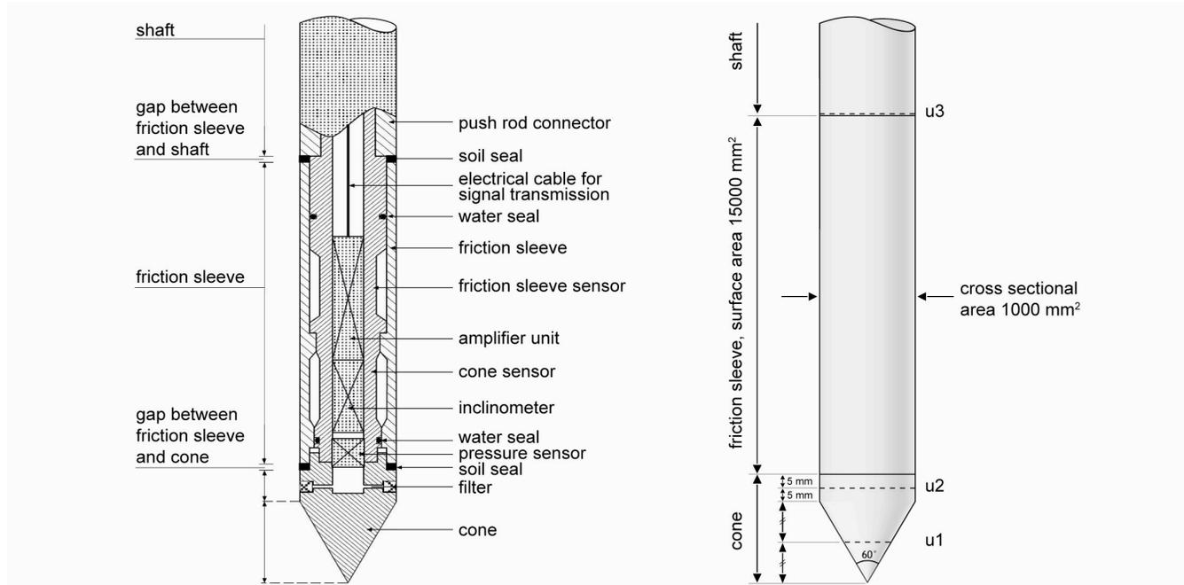
Figure 2. Example cone penetrometer from practice and proposed cone penetrometer for Analytic CPT.
