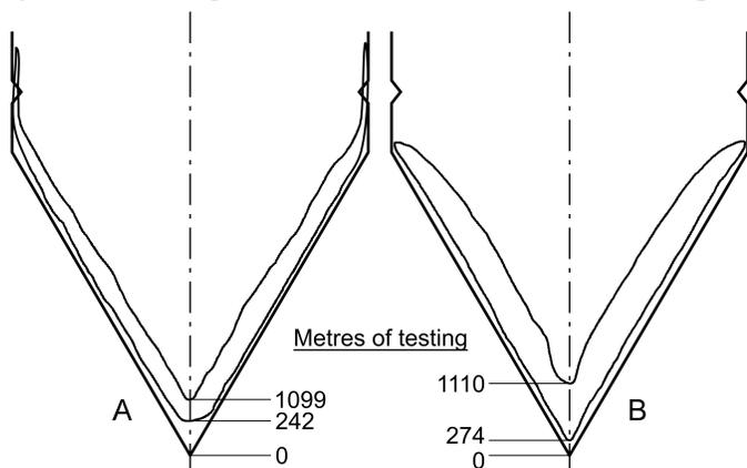
Figure 3. Wear of cones made of different materials after approximately same metres of penetration (Schaap & Zuidberg 1982).
