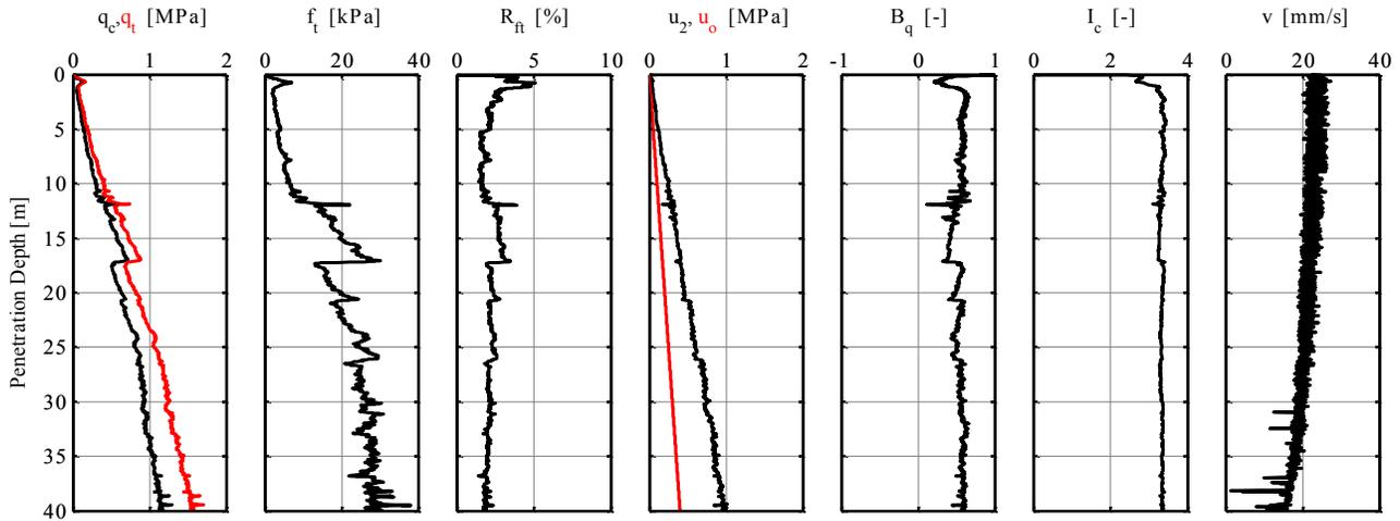
Figure 21. Unusual reduction in  $q_t$  and  $f_t$  at 17 m penetration depth.
