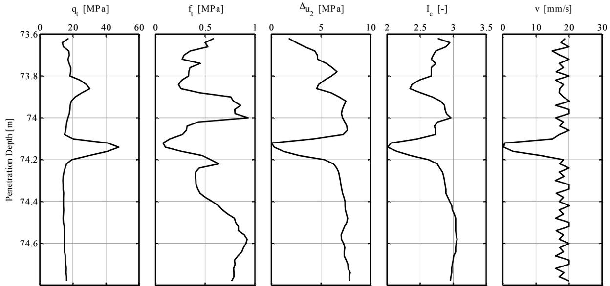
Figure 15. Example of penetration rate affecting CPT parameters for chalk (Peuchen & Balthes 2013).
