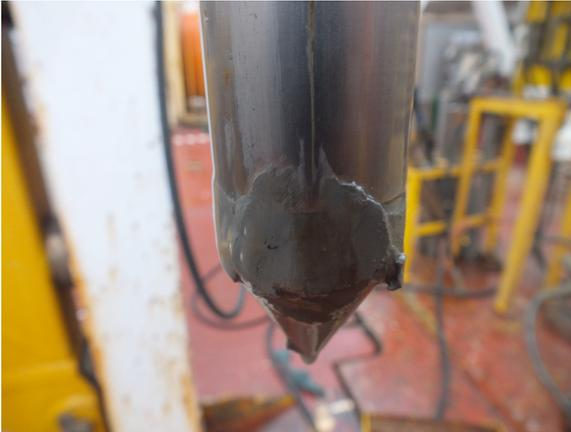
Figure 5. Clay adhering to cone penetrometer after retraction from soil.
