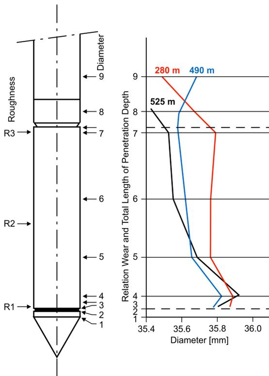
Figure 10. Observed geometry after wear (in sand) of three different cone penetrometers (Jekel 1988).
