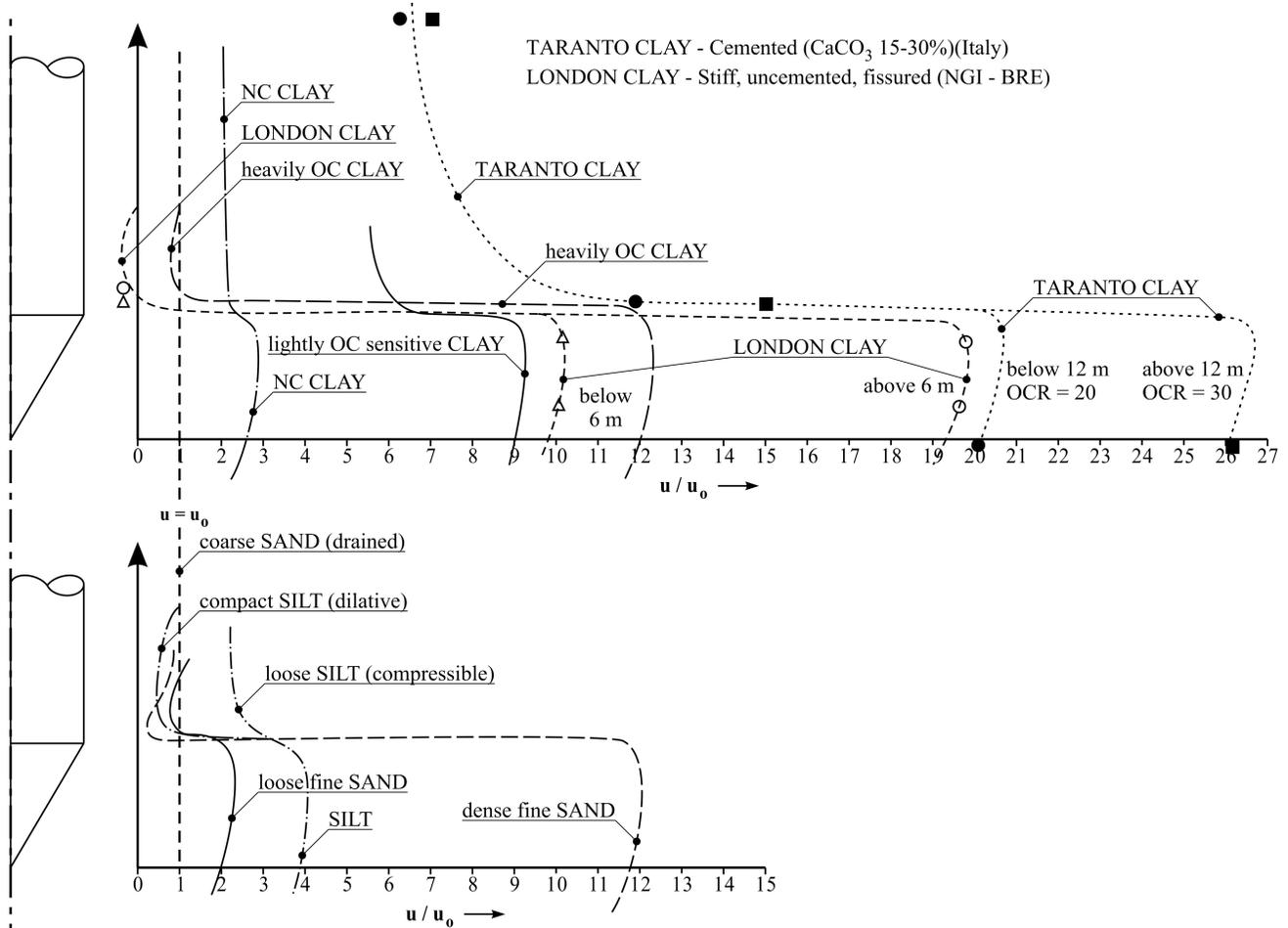
Figure 13. Pore pressure distribution in saturated soil (adapted from Robertson et al. 1986).
