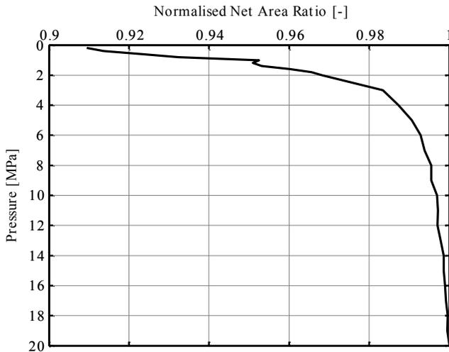
Figure 4. Laboratory water pressure versus normalised net area ratio.
