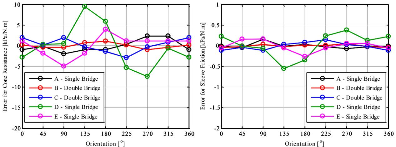
Figure 7. Measurement error due to bending moment - cone resistance (left) and sleeve friction (right).
