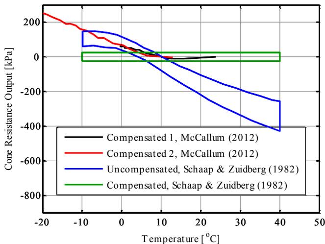
Figure 9. Zero drift of cone load cell caused by ambient temperature change.
