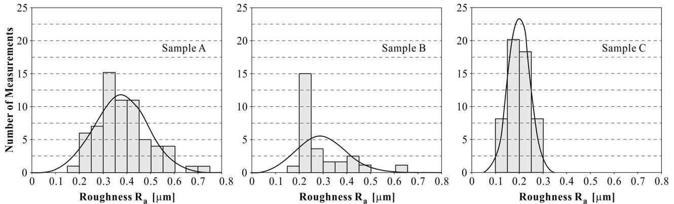
Figure 11. Surface roughness of friction sleeves observed after use (Schaap & Zuidberg 1982).
