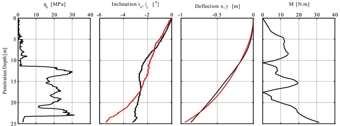
Figure 6. Bending moment inferred from cone penetrometer inclination.
