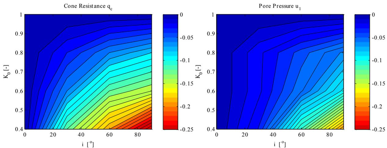
Figure 17. Influence of non-vertical trajectory on cone resistance  $q_c$  (left) and pore pressure  $u_1$  (right), expressed as fraction of  $K_0 = 1$  and  $i = 0^\circ$  (scale for colour bars is 0 to -0.25), after Wei et al. (2005).
