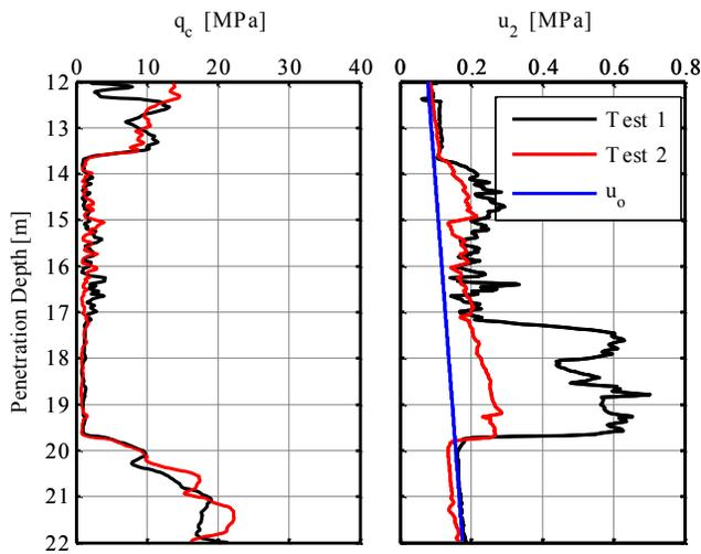
Figure 12. Pore pressure response for two closely spaced CPTs.
