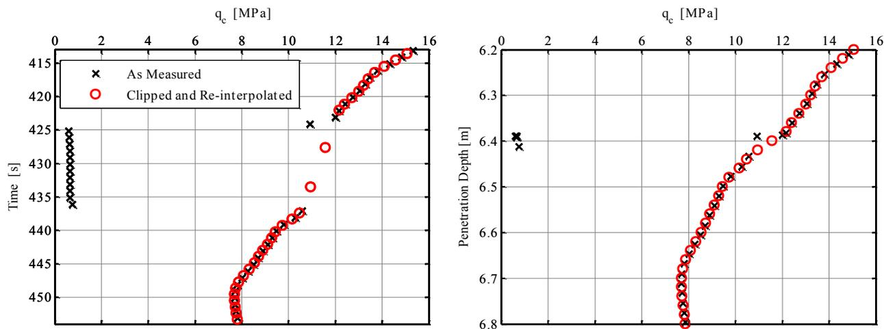
Figure 16. Penetration interruption - cone resistance  $q_c$  versus time (left) and  $q_c$  versus penetration depth (right).
