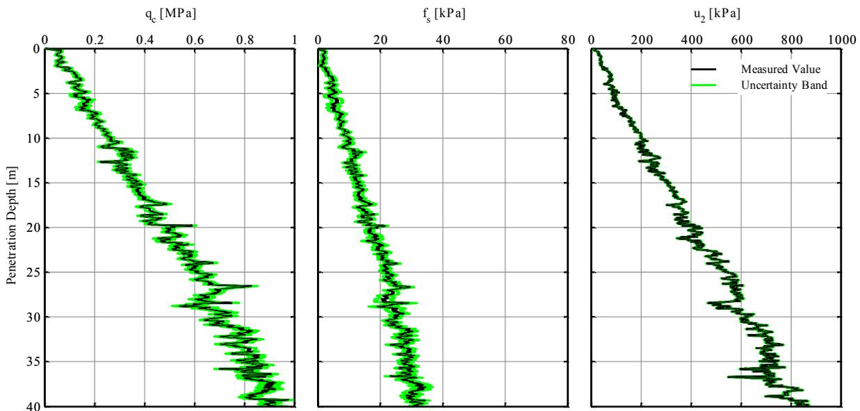
Figure 18. Uncertainty estimates according to ISO 22476-1 for CPT values measured under favourable conditions of homogeneous slightly overconsolidated clay.
