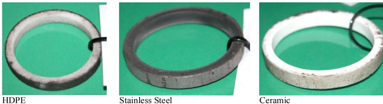
Figure 14. Filter elements ( $u_2$ ) after use.
