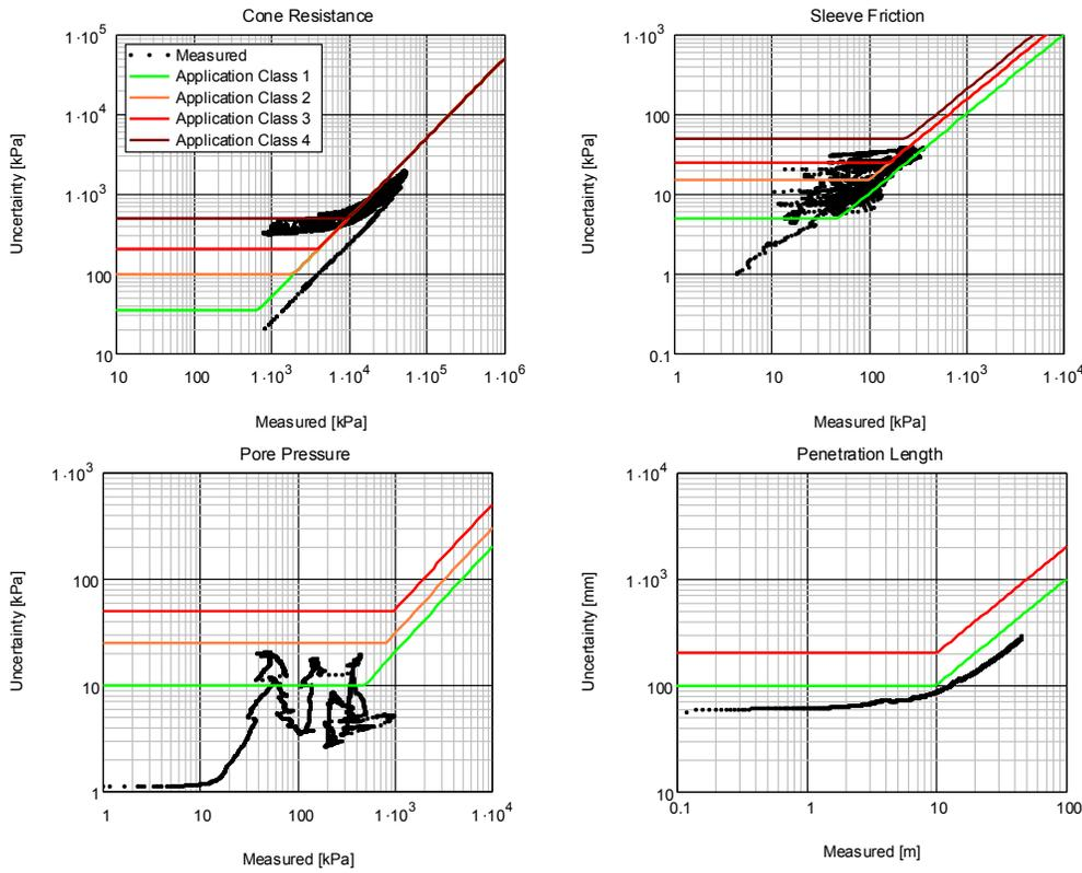
Figure 19. Uncertainty estimates according to ISO 22476-1 for CPT values measured under adverse conditions of layered sands and clays.
