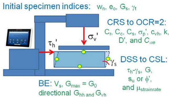
Figure 19. Conceptual all-in-one hybrid laboratory test
