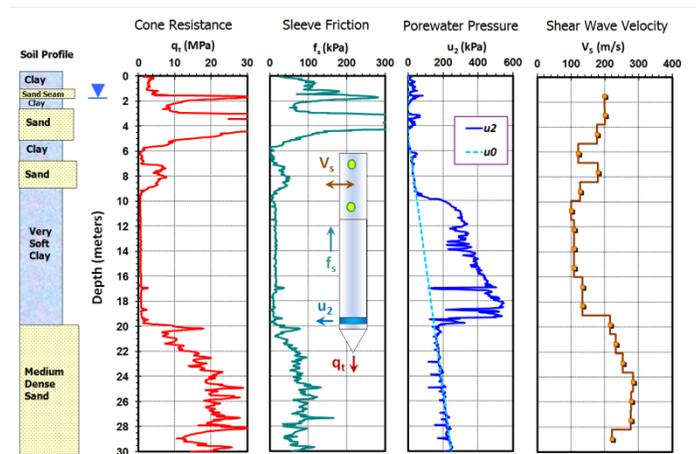
Figure 18. Representative seismic piezocone sounding from New Orleans East, Louisiana
