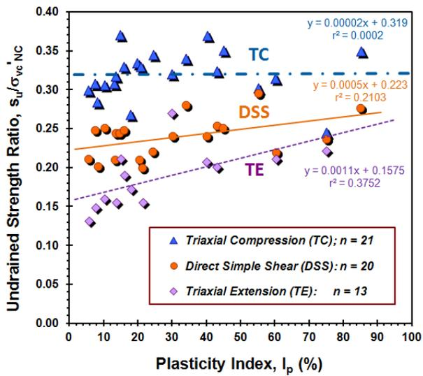
Figure 11. Strength ratio vs PI for clays tested in triaxial compression, simple shear, and extension modes (Ladd 1991)
