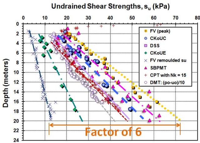
Figure 6. Family of  $s_u$  profiles from various tests in Bothkennar clay, UK (after Hight et al. 2003)
