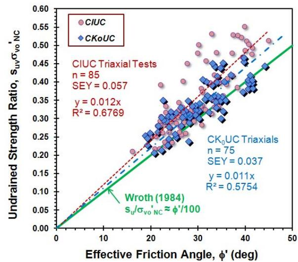
Figure 9. Trends of triaxial strength ratio ( $S$ ) with effective  $\phi'$  for many clays tested under CIUC and  $CK_0UC$
