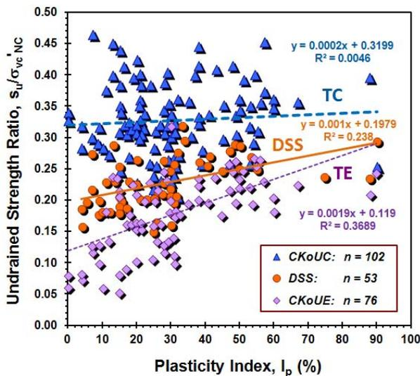
Figure 12. Database trends for strength ratio vs PI for clays tested by CK<sub>0</sub>UC, DSS, and CK<sub>0</sub>UE modes
