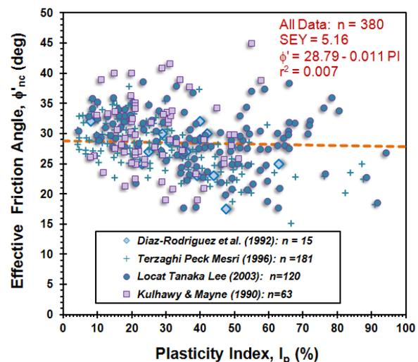
Figure 10. Lack of correlation between  $\phi'$  and PI in clays
