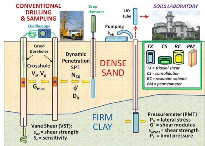
Figure 3. Comprehensive all-out program for geotechnical site characterization using in-situ, laboratory, and geophysics
