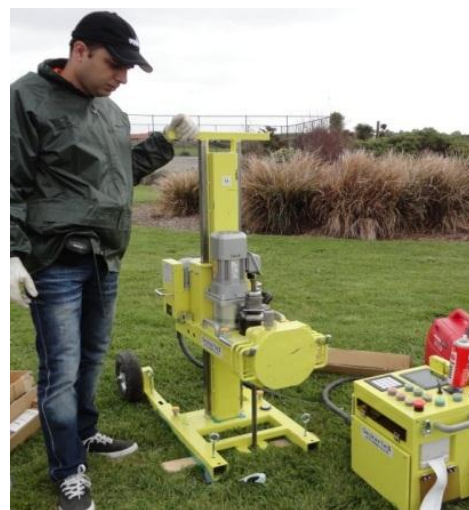
Figure 2 SDS machine during operation
